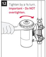
Only use Silicon grease or water to lubricate O ring.
