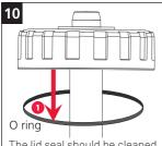
The lid seal should be cleaned and checked for wear when servicing MagnaClean. It is Best Practice to replace the lid seal at each service.
