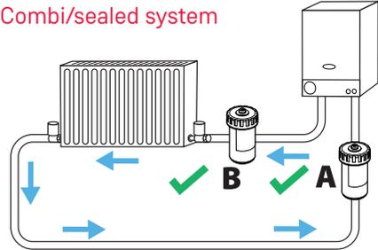
Note: In both diagrams, position A is best practice, Position B is suitable if space is tight on the return.
