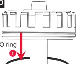
The lid seal should be cleaned and checked for wear when servicing *MagnaClean*. It is Best Practice to replace the lid seal at each service.
