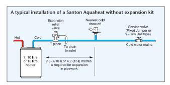
For installations where any of the above conditions cannot be met, an expansion vessel and other relevant accessories must be used to accommodate expansion.
