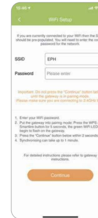
**8.** Press and hold the WPS/Smartlink button in the back of the gateway until the green WiFi light begins to flash, quickly press the continue button on the Ember app.
