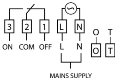
\* If mains voltage output is required, terminals L & 2 must be electrically linked.
