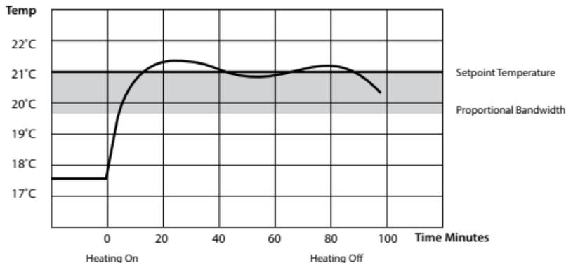
*Example: Program 1 on the thermostat is 21°C for 06:30am and the room temperature is 18°C. The thermostat will start the heating at 06:30am and the room temperature will start to increase then but will switch itself off before it reaches temperature and allow the room temperature to increase naturally – this cycle may begin again if the thermostat isn't reaching temperature.*
