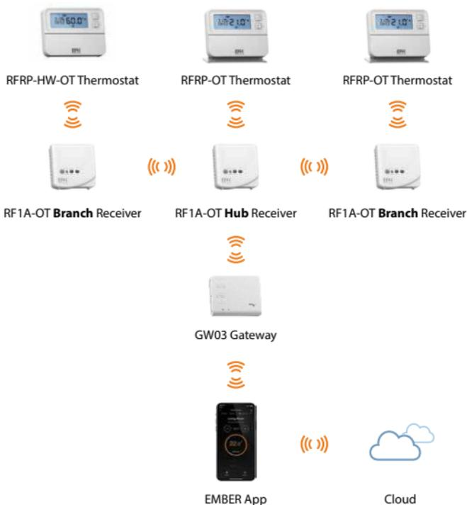
Note: A maximum of 6 thermostats can be used in the system.
