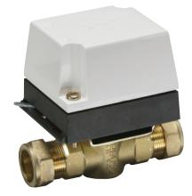
The H-Series Motorised Valves, working in conjunction with time controls and thermostats, are used in domestic and commercial central heating, hot water and chilled water systems to control the flow of water in the system.
